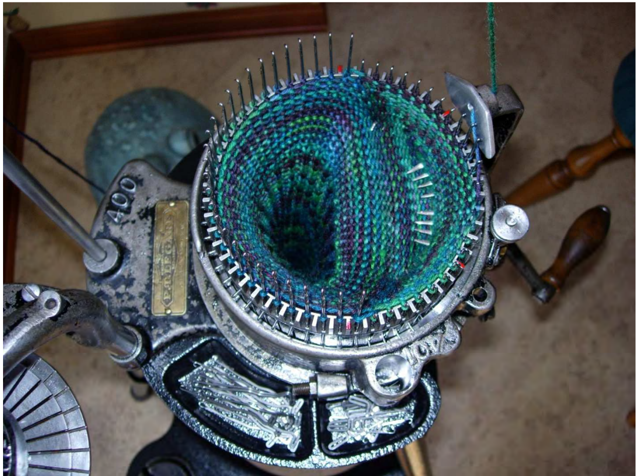
Newer Legare 400 Oval Base (note adjuster screws on gear ring)
