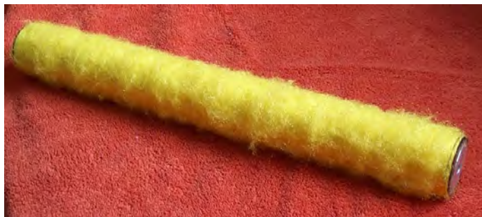
Very soft roller for cleaning or transporting film.
