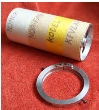
Yarn drum with simple tool for compacting single layer.
