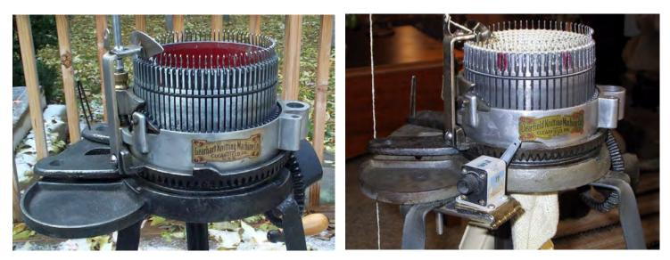
Compare the Gearhart Machine on the left with the Clearfield Machine on the right. The machines look identical, although the rear leg under the Clearfield appears to be attached at a different location.
