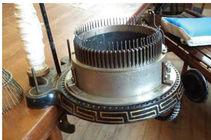
View of left side. Note a series of holes around the base. These hole were for pins that served to stop the carrier and shift the cams into reverse when turning a heel or knitting flat web.
