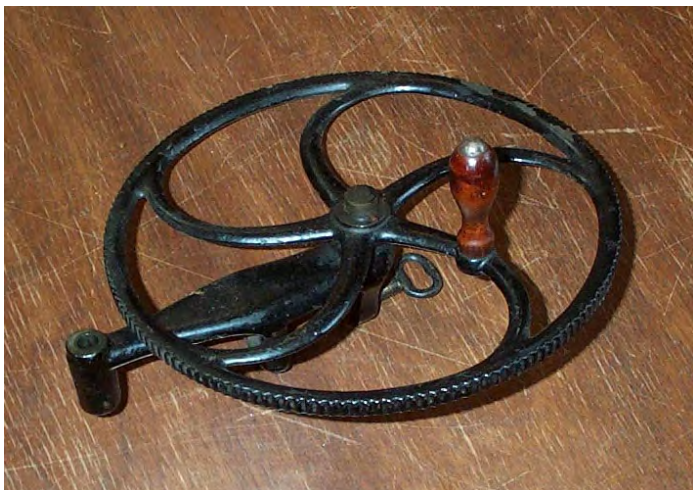
Bickford Bobbin Winder . The wheel contacted a rubber roller, not shown.
