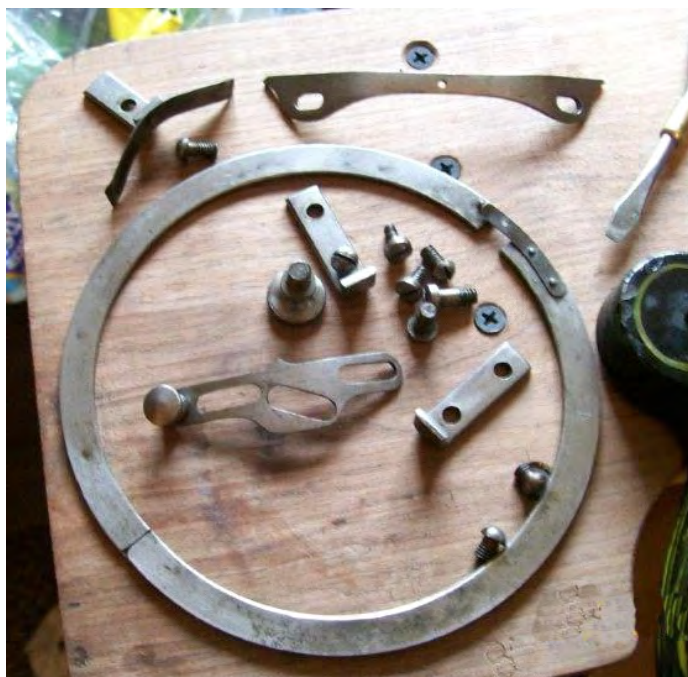
Figure 5. The large ring here is the Ring Clasp . It holds needles in the Needle Cylinder , and also holds the Revolving Cam Ring down against the Bedplate .
