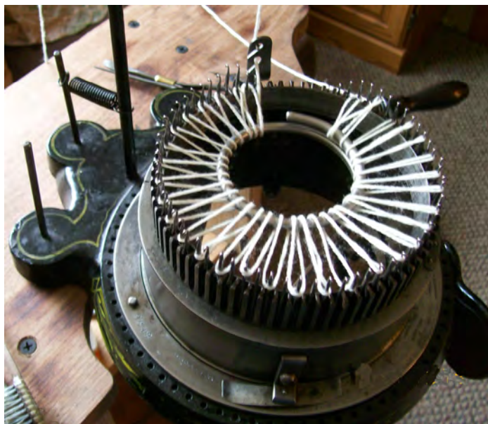
Figure 9. Setting up the Bickford for tubing.
