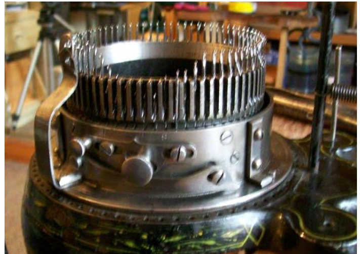
Figure 2. Carrier on the left. Left end of Automatic Lever is up.
