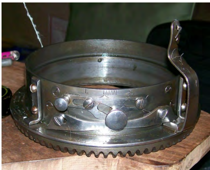
Figure 11. View of cam controls. These controls adjust stitch length and reverse the cams. The Automatic Lever was also shown in Figure 3. The right end is resting on the carrier pad.
