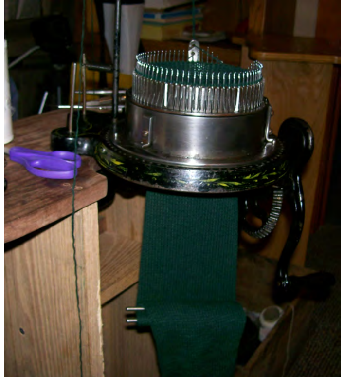
Figure 12. Sixty inches of yarn tubing was done with no dropped stitches.
