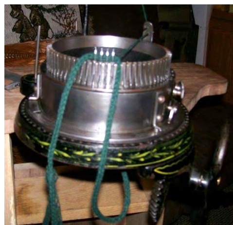
Figure 7. The carrier must be slightly more than a quarter inch from the needles to avoid breaking latches. The delayed timing of the carrier is just right for feeding yarn to the needles.
