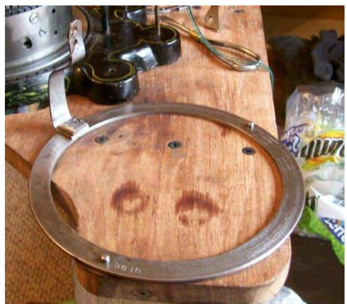
Figure 4. The carrier is shown here mounted on the Sliding Ring . Note two short pegs on the Sliding Ring . They limit how far the carrier will move when changing direction of rotation.
