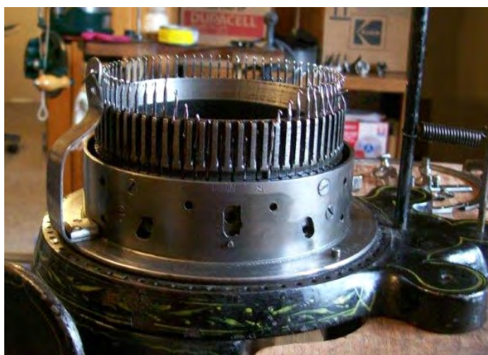
Figure 6. This shows the Revolving Cam Ring striped of all screws and external parts. The Yarn-Carrier and Sliding Ring assembly can be lifted off the machine in this configuration, without removing the needles or Revolving Cam Ring .
